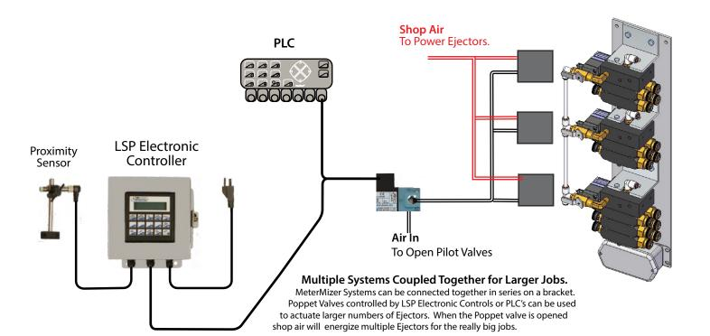
Maintain air pressure entering the Manual Valve or the Solenoid Valve at 60 to 80 PSI
