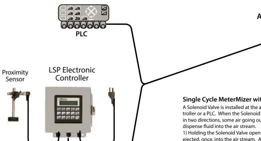
The LSP Electronic Controller Can be programmed on a count pulsating or timer sequence.. Controller will receive a signal from the Proximity Sensor or from a limit switch tied into an operating machine. See catalog for deferent controllers.
