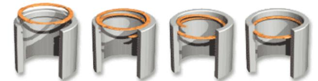
2. Insert three RETURN SPRINGS(21) into BARREL(1). Put a SPRING GUIDE(22) into each.
